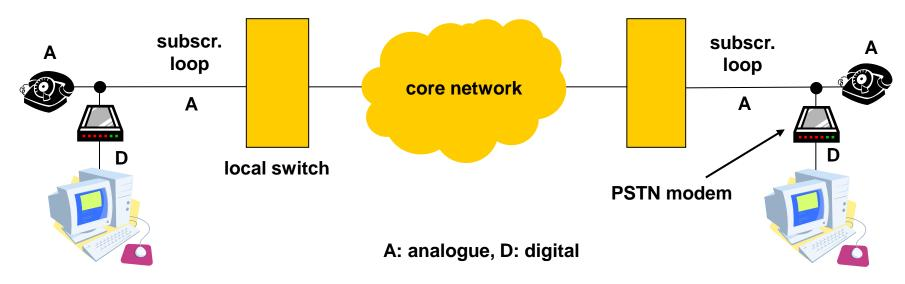
While the core network was analogue, the D/A, A/D converting function of the modem was necessary
