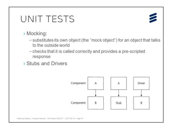
*Mock objects* are a popular tool for isolating classes for unit testing. When using mock objects, your test
