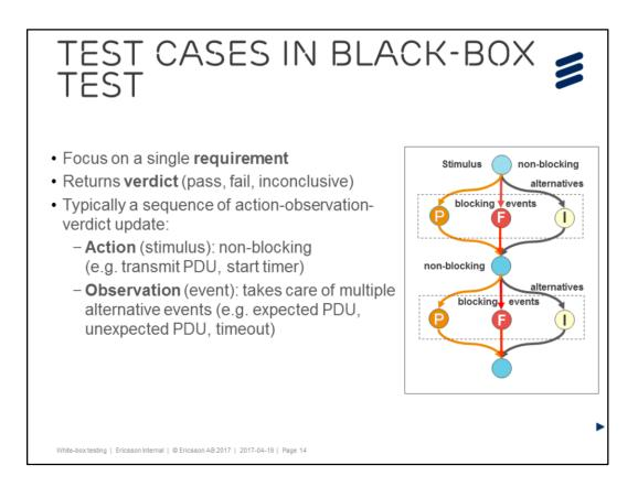
**Black-box** testing means that the internal structure of the tested software product is not known: the only way to test it is to send a message ("stimulus") to the system and to analyse the received response. The latter is compared to the due response determined beforehand using the reference specification. If the comparison ("pattern matching") between the real and the expected response fails, the test case is considered as "failed" otherwise "passed".
