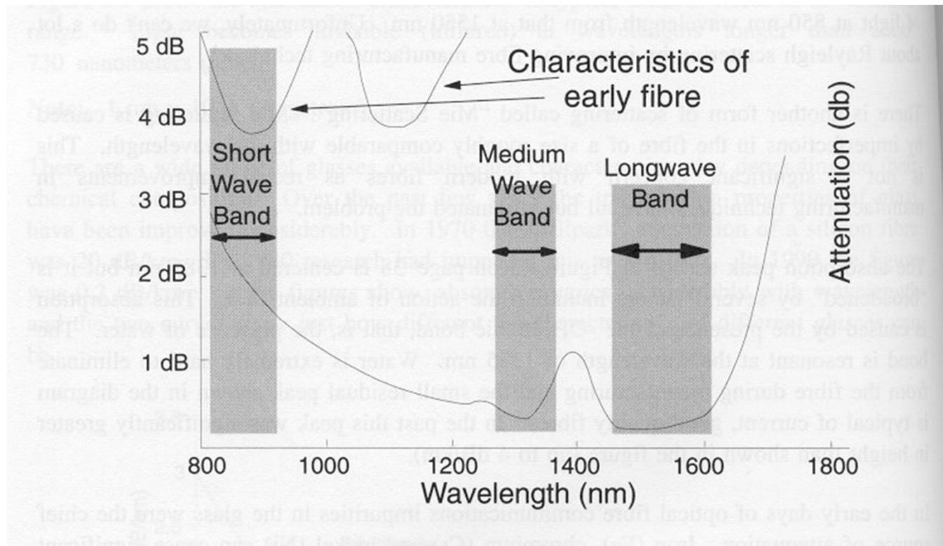
**Figure 14.** Transmission Windows. The upper curve shows the absorption characteristics of fibre in the 1970s. The lower one is for modern fibre.
