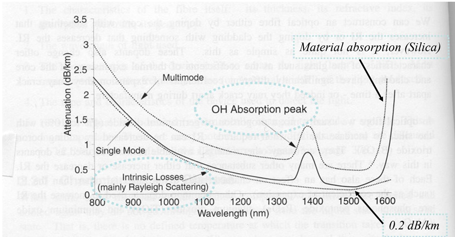
**Figure 13.** Typical Fibre Infrared Absorption Spectrum. The lower curve shows the characteristics of a single-mode fibre made from a glass containing about 4% of germanium dioxide ( $\text{GeO}_2$ ) dopant in the core. The upper curve is for modern graded index multimode fibre. Attenuation in multimode fibre is higher than in single-mode because higher levels of dopant are used. The peak at around 1400 nm is due to the effects of traces of water in the glass.
