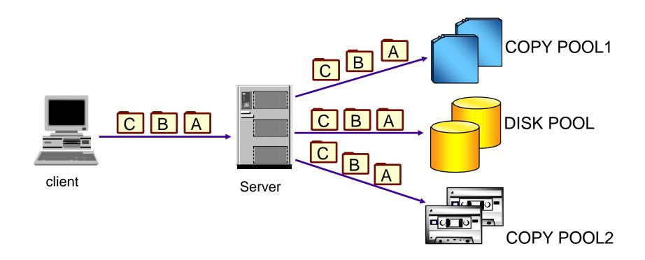
More back-up storage pools can be defined, simultaneous writing The target storage pools can be of different types (tape, disk). Disaster tolerant systems
