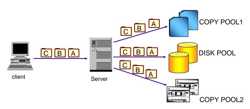
More back-up storage pools can be defined, simultaneous writing The target storage pools can be of different types (tape, disk). Disaster tolerant systems
