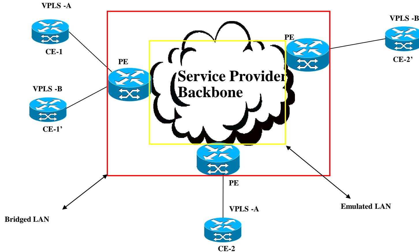
Customer Edges (CE): Client side device, typically Ethernet
