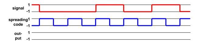
8. Decode the following signal with the given spreading code!
