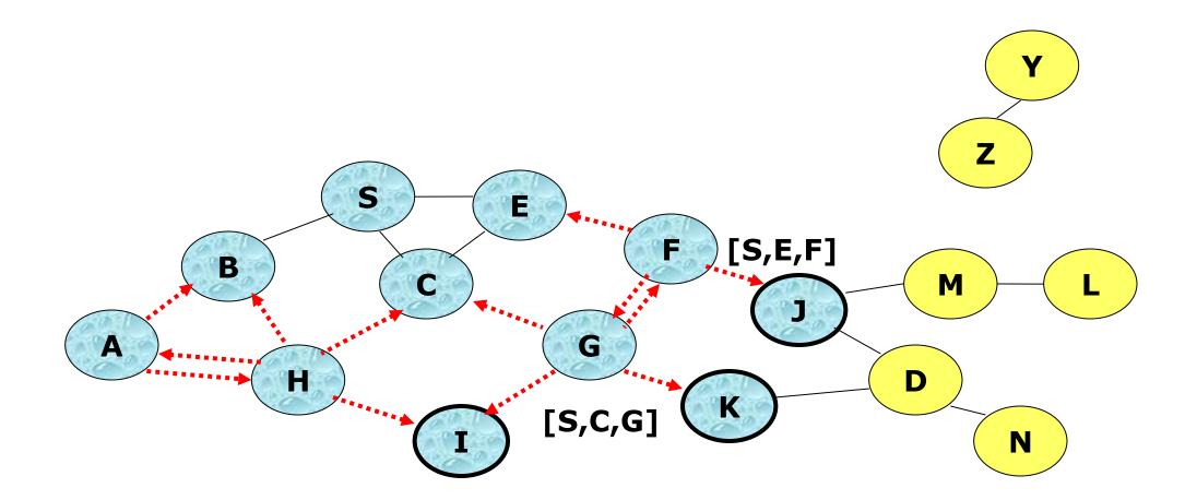
Restricting the flooding (like in AODV): C receives the RREQ again from G and H, but does not forward it again
