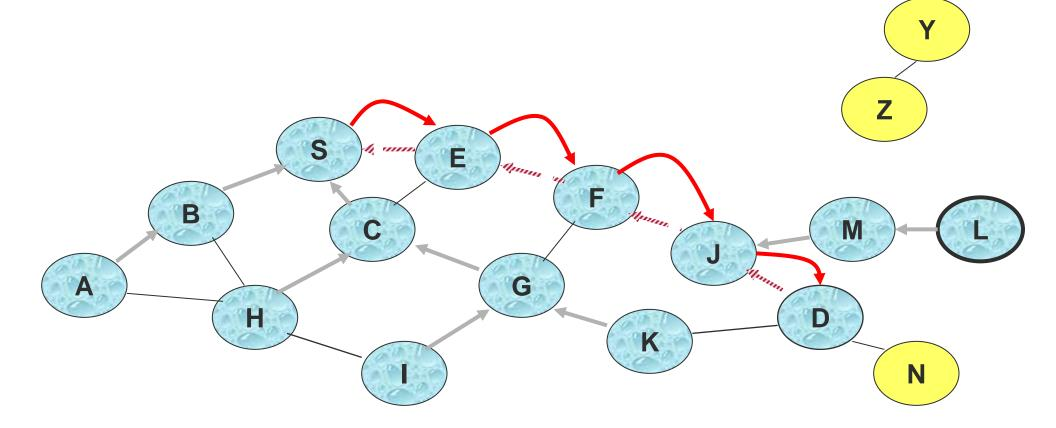
As the RREP message travels from D to S, forward path pointers are stored in the intermediate nodes
