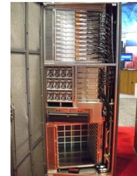
2011: Fujitsu K computer rack, Kobe, Japán (10 petaflops)
